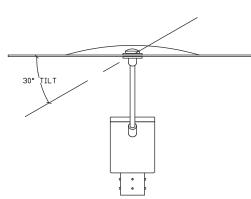
Top: aluminum disk with spun aluminum parabolic domed reflector, with two ball joints for 30 tilt. Top is supported with two s/s rods.
