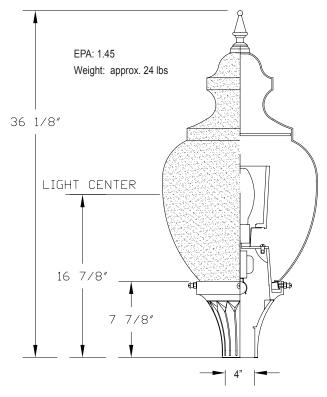
The SH01 series square luminaire shall consist of a top finial, "acorn" diffuser, capital, ballast assembly and an internal optical system. The diffuser shall be either clear stippled acrylic or polycarbonate or opal white polycarbonate. The capital (fitter) shall be cast aluminum. All castings shall be formed true to pattern, with no warping or mold shifting.
