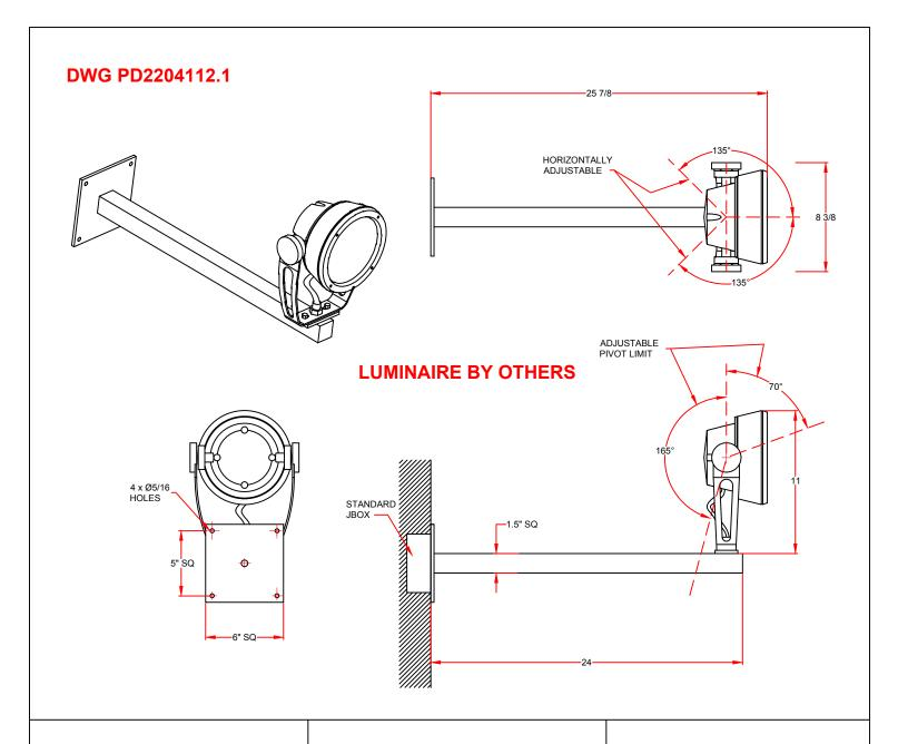
**Luminaire: BY OTHERS.** Note: this mounting arm is designed specifically for the Lumenpulse Lumenbeam LMB luminaire.
